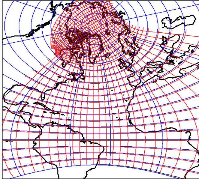
The model domain was built with horizontal resolution of  $1 \times 1^\circ$  in Atlantic. The reprojected bipolar grid in Arctic has minimum spacing equal to 35km while maximum spacing is about 62km.
